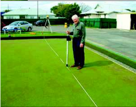
Surveying to check levels.
